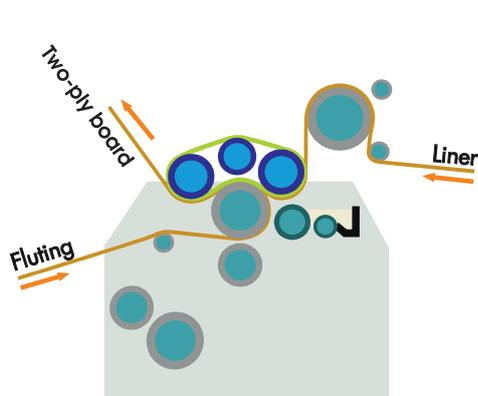
Fig. 7. Single facer with a pressure belt
