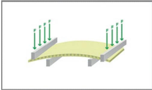
Fig. 33. Bending stiffness test
