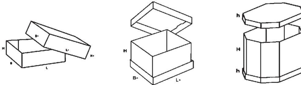
Fig. 13. Telescope-type boxes – examples
