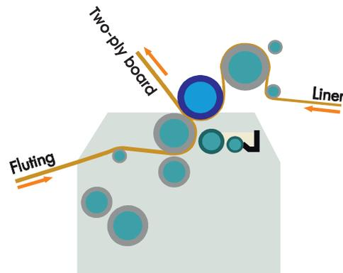
Fig. 8. Single facer with a pressure roll
