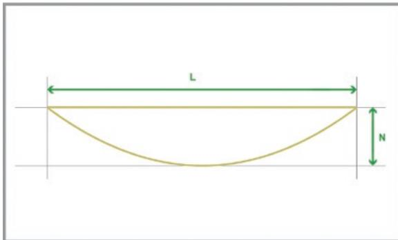
Fig. 35. Corrugate board flexion
