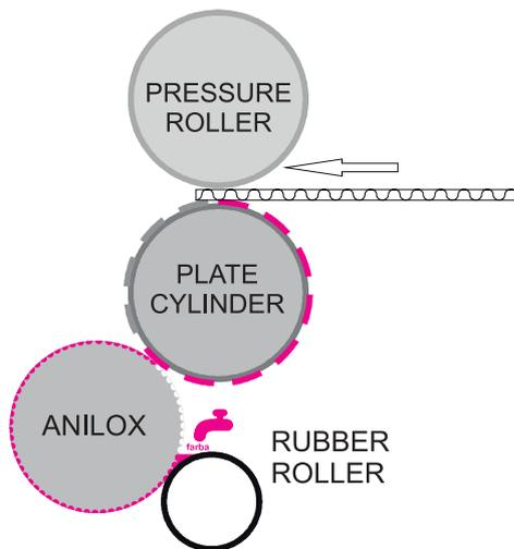
Fig. 22. Diagram of a flexographic printer with a rubber roller
