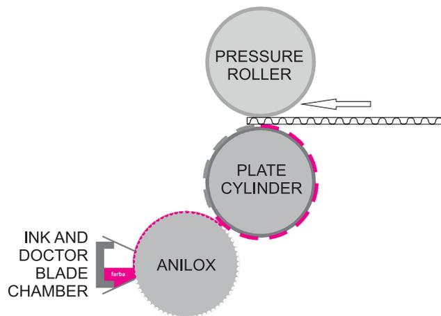
Fig. 21. Diagram of the flexographic printer with the ink and doctor blade chamber
