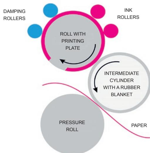
Fig. 29. Diagram of an offset printer
